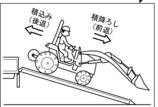
Please use reverse gear when getting on the truck. Use the forward gear when getting off the truck
